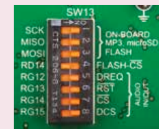
Figure 14-2: Enabling audio codec communication lines
