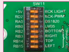
Figure 21-3: Enabled SW11.4 DIP switch
