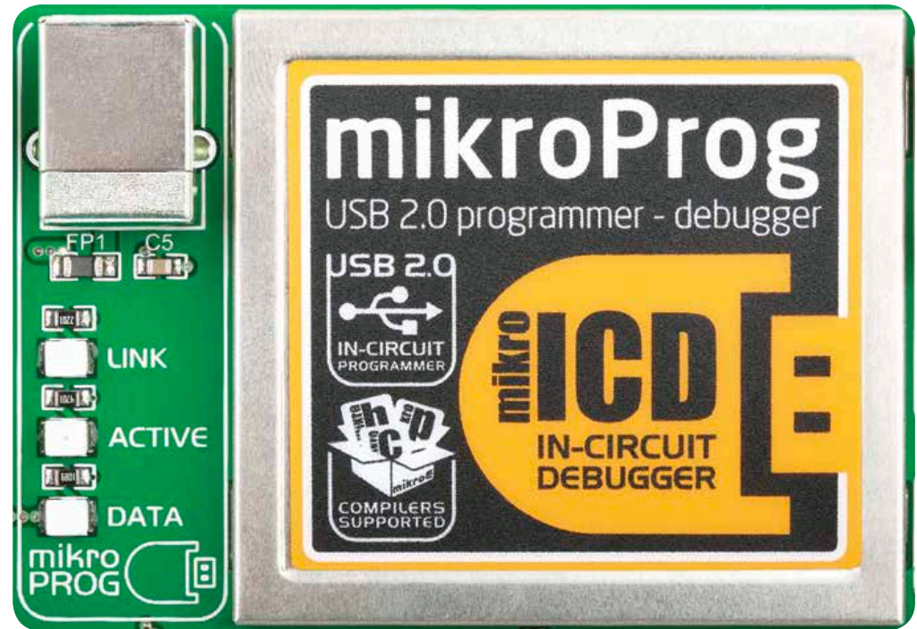
Figure 5-1: mikroProg™ is well protected under metal casing
