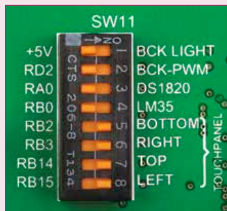
Figure 17-2: Turn on switches 5 through 8 on SW11 to enable Touch panel controller
