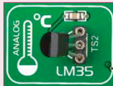
Figure 21-2: LM35 correctly placed in socket
