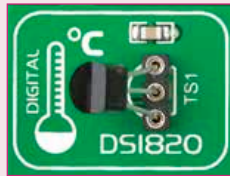
Figure 20-2: DS1820 correctly placed in socket
