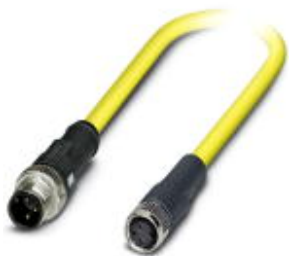
Sensor/Actuator cable, 3-position, PVC, yellow, Plug straight M12 SPEEDCON, A-coded, on Socket straight M8, Cable length: 0.5 m
