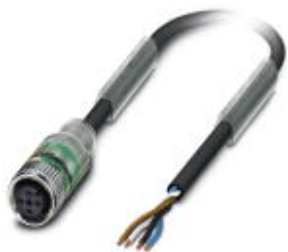
Sensor/actuator cable, 4-position, Variable cable type, free cable end, on Socket straight M12, A-coded, with 2 LEDs, cable length: Free input (0.2 ... 40.0 m)
