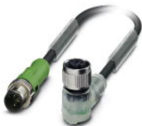
Sensor/actuator cable, 3-position, Variable cable type, Plug straight M12 SPEEDCON, A-coded, on Socket angled M12 SPEEDCON, A-coded, with 2 LEDs, PIN 2+4 bridged, cable length: Free input (0.2 ... 40.0 m)
