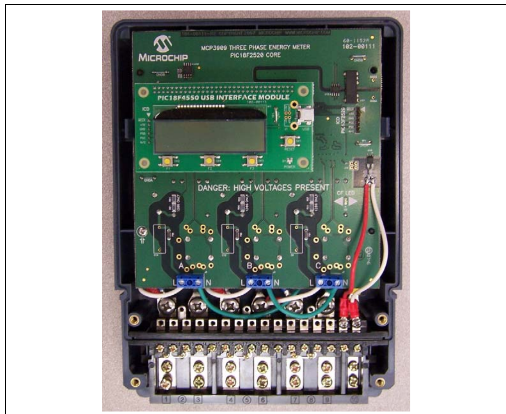
FIGURE 1-1: MCP3909 3-Phase Energy Meter Reference Design.
