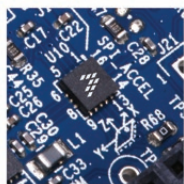
Freescale Freedom Development Platform featuring the SPI Accelerometer
