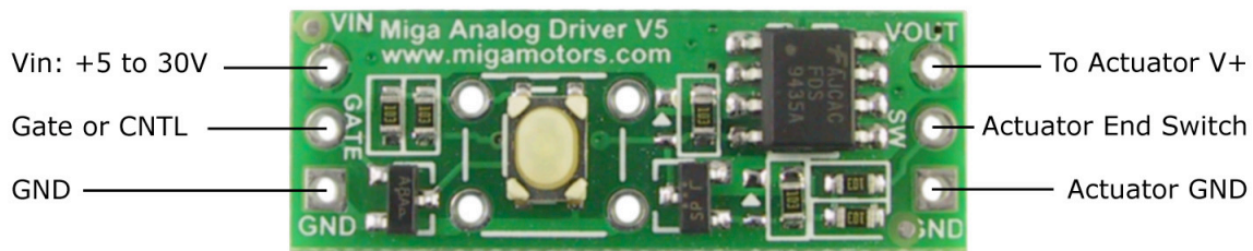
Miga Analog Driver V5 -Pinout Diagram
