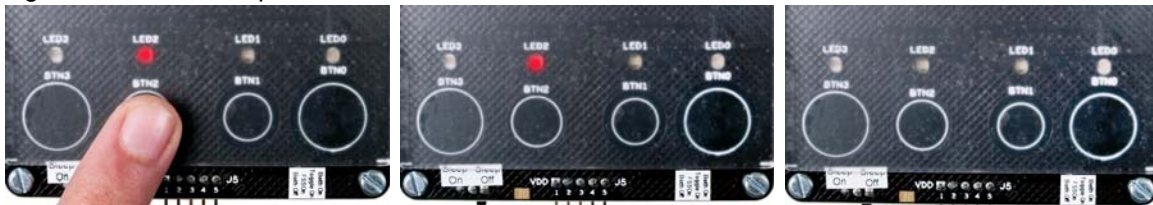
Figure 3-15. Test Sequence for LED On Time Feature
