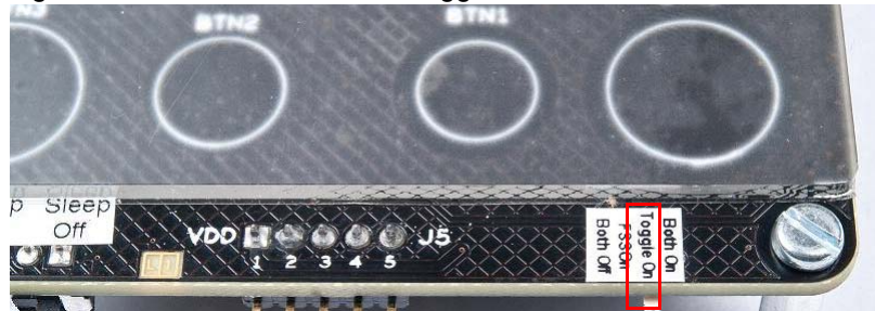
Figure 3-3. Switch Position for Toggle Feature
