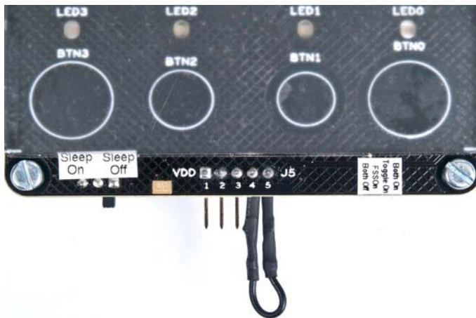
Figure 3-22. BTN1 Sensor Shorted to Ground
