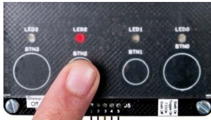
1. Touch a button; the LED turns on
