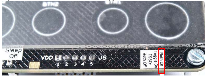
Figure 3-11. Switch Position for Toggle and FSS Features
