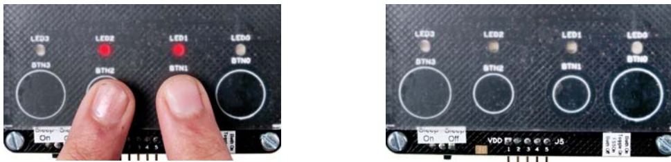
Figure 3-10. Kit with Toggle and FSS Features Disabled
