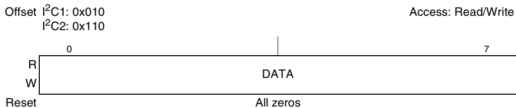
Figure 11-6. I 2 C Data Register (I2CDR)
