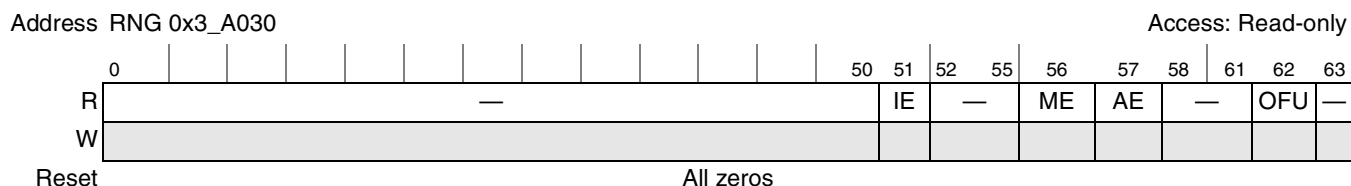
Figure 12-44. RNG Interrupt Status Register
