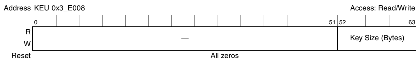
Figure 12-58. KEU Key Size Register
