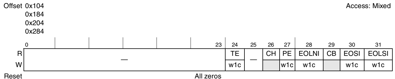
Figure 16-5. Status Registers (SRn)
