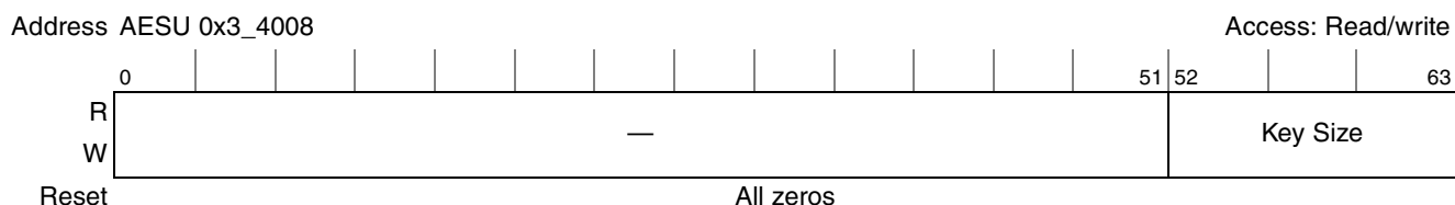
Figure 12-48. AESU Key Size Register
