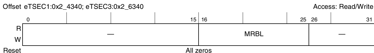
Figure 15-31. MRBLR Register Definition
