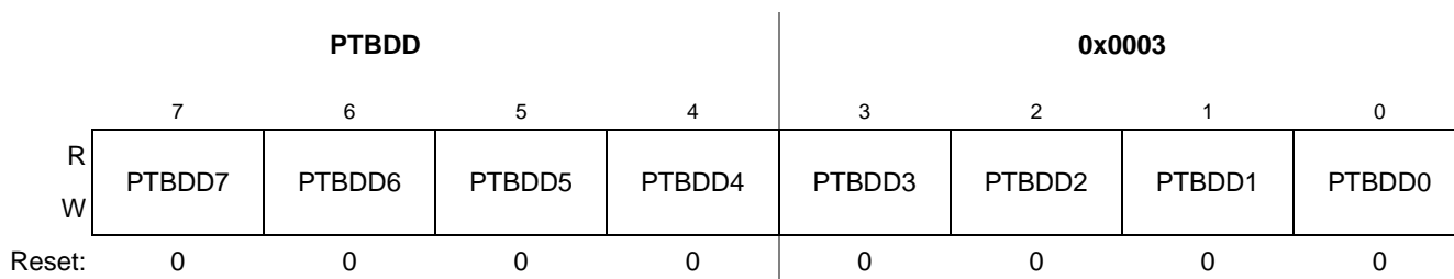
Figure 9-8. Port B Data Direction Register (PTBDD)
