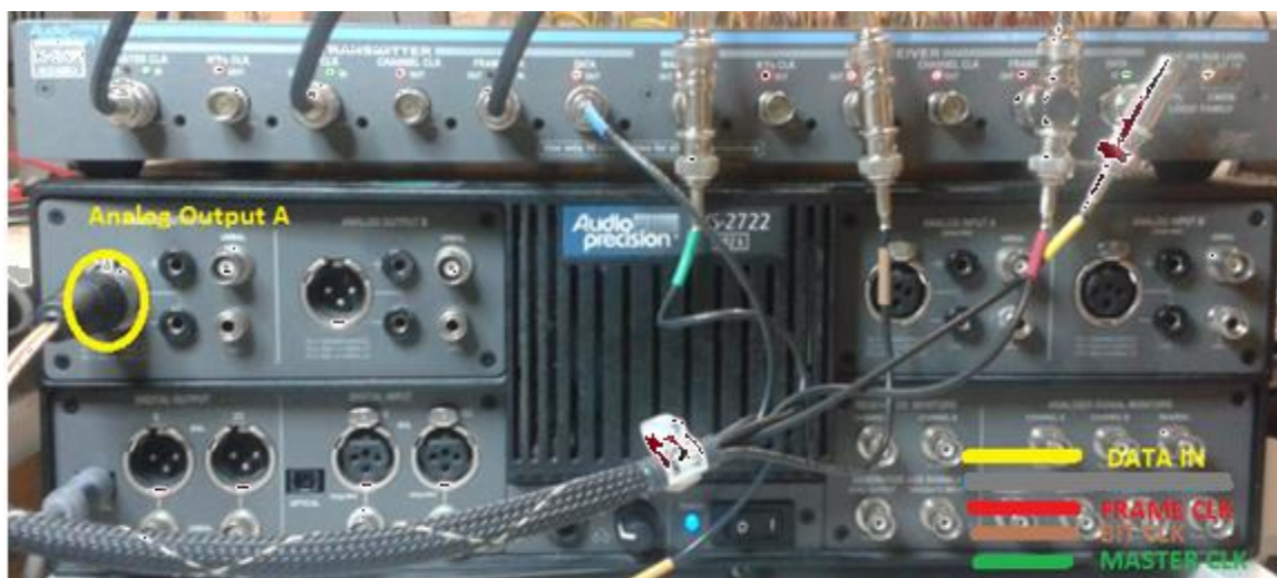
Figure 8: AP connection for NAU85L40 ADC
