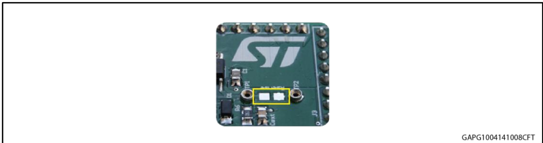
Figure 5: Pads for soldering SMD resistor
