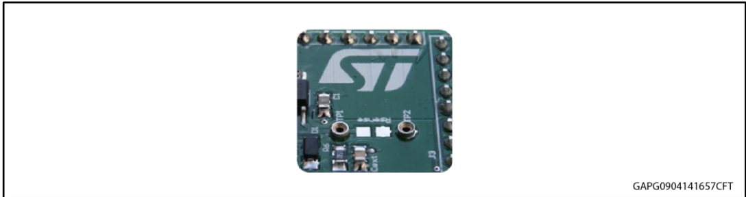
Figure 4: Mounting through-hole sense resistor
