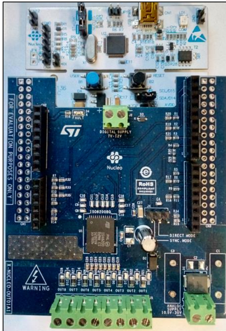
Figure 2: X-NUCLEO-OUT01A1 plugged on an STM32 Nucleo board
