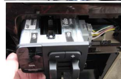
Brake Controller Slides Out
