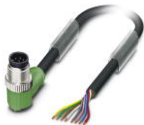
Sensor/actuator cable, 8-position, Variable cable type, Plug angled M12, A-coded, on free cable end, cable length: Free input (0.2 ... 40.0 m)
