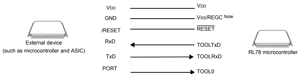
Figure 25 - 4 Communication with External Device
