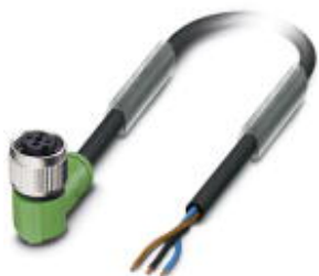
Sensor/actuator cable, 3-position, PUR halogen-free, black-gray RAL 7021, free cable end, on Socket angled M12 SPEEDCON, A-coded, cable length: 5 m
