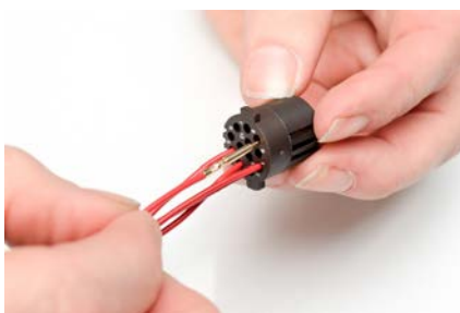
Step 4 - Push wire into insert
