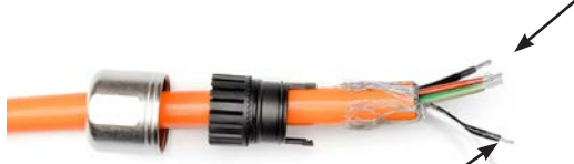
Step 5b - Strip signal wire 4.5mm
