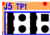
Figure 3: Shows the voltage selection jumpers
