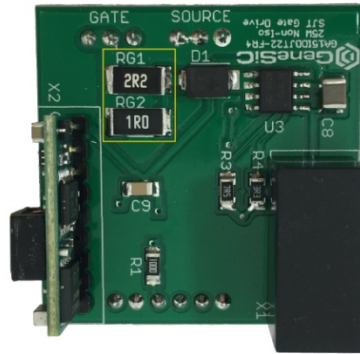
Figure 5: Location of R_G (RG1 and RG2 in parallel) on GA15IDDJT22-FR4 driver for substitution
