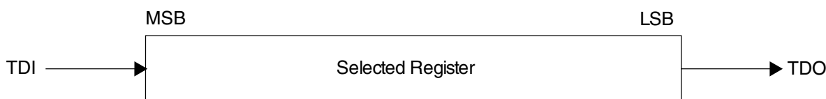
Figure 45-3. Shifting data through a register
