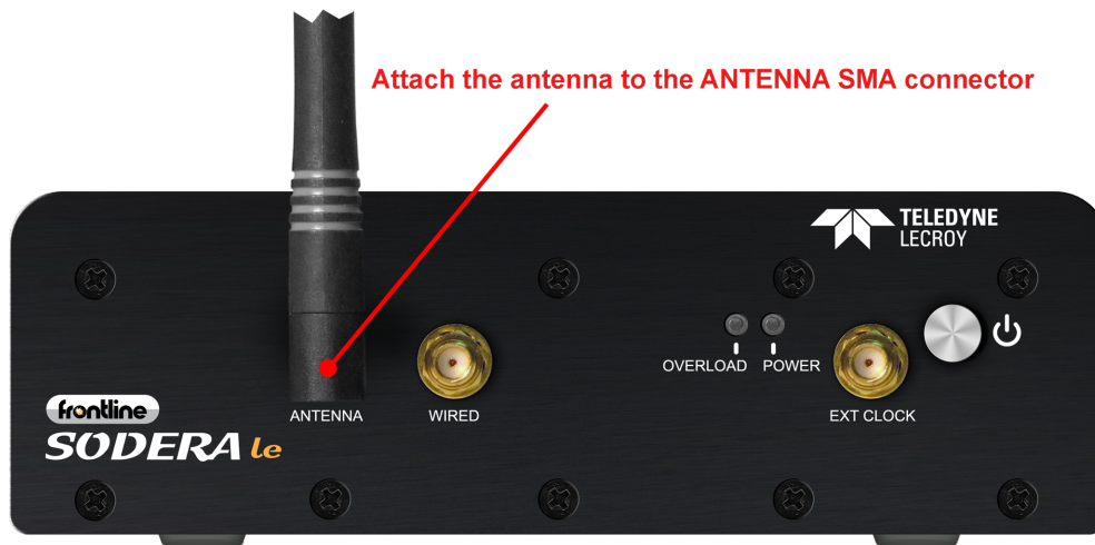
Figure 2.3 - Antenna Attachment Point
