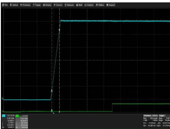
Figure 5: CSU550AP-3 Output Voltage Startup Characteristic – Vin = 90Vac Full Load: I_o = 45A , I_{SB} = 2.5A Ch 3: V_o Ch 4: PWOK
