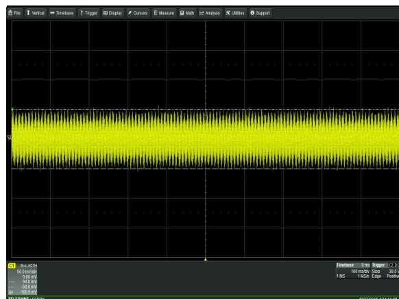
Figure 6: CSU550AP-3 Ripple and Noise Measurement – Vin = 90Vac Full Load: I_o = 45A , I_{SB} = 2.5A Ch 1: V_o
