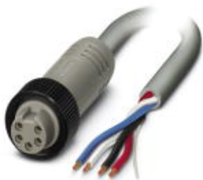
Bus system cable, DeviceNet™, 5-position, PVC, gray, free cable end, A - standard, on Socket straight 7/8"-16UNF, A - standard, cable length: 20 m
