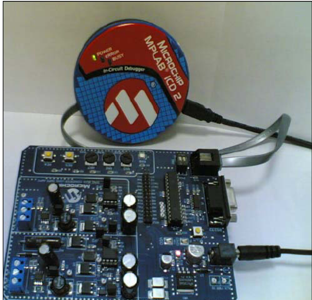
FIGURE 3-12: dsPICDEM™ SMPS BUCK DEVELOPMENT BOARD CONNECTED TO MPLAB® ICD 2 IN-CIRCUIT DEBUGGER
