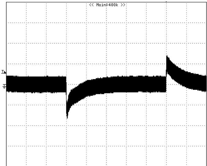
Figure 19: Typical transient response to step load change at 1A/μS from 100%~ 50%~100% of Io, max at 12Vin, 5.0Vout (Cout = 1uF ceramic, 47uF+10μFceramic) CH1 : VOUT, 50mV/div, 200uS/div
