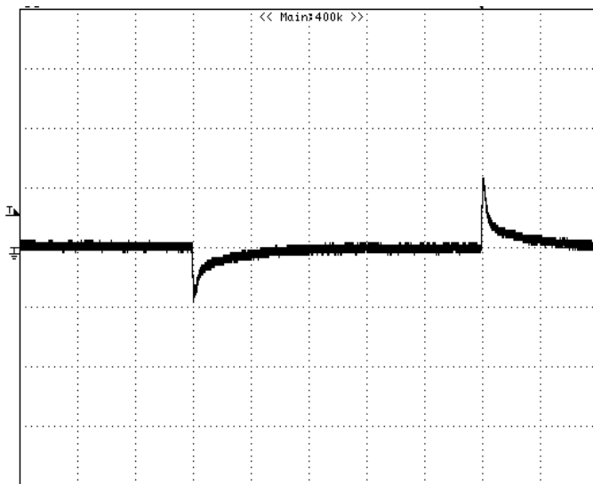
Figure 24: Typical transient response to step load change at 1A/\mu S from 100%~ 50%~100% of I_o , max at 12V_{in} , 0.59V_{out} ( C_{out} = 1\mu F + 47\mu F + 10\mu F ceramic) CH1 : VOUT, 50mV/div, 200uS/div
