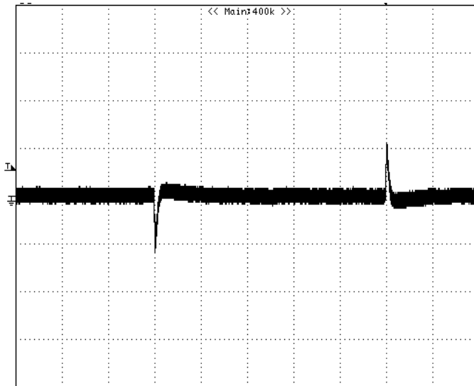
Figure 22: Typical transient response to step load change at 1A/\mu S from 100%~ 50%~100% of I_o , max at 12V_{in} , 1.8V_{out} ( C_{out} = 1\mu F + 47\mu F + 10\mu F ceramic) CH1 : VOUT, 50mV/div, 200uS/div
