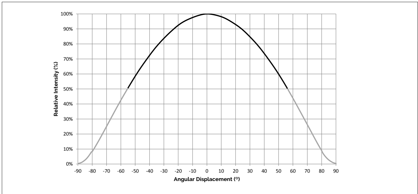
Figure 10: Typical Spatial Radiation Pattern
