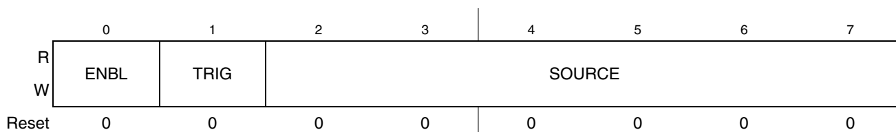
Figure 22-2. Channel Configuration Registers (CHCONFIGx)
