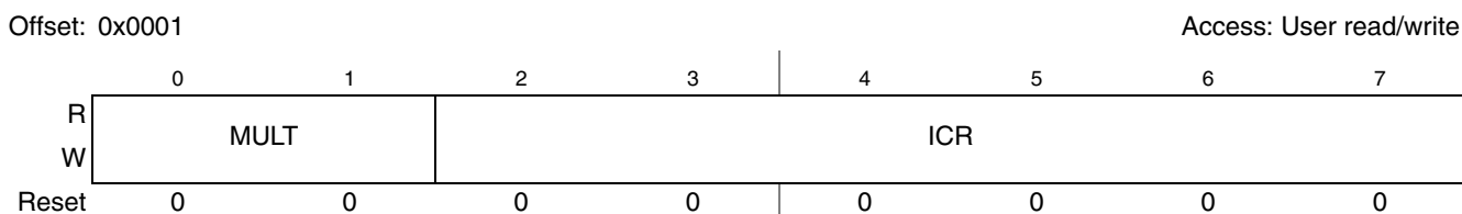
Figure 31-4. I 2 C Bus Frequency Divider Register (IBFD)
