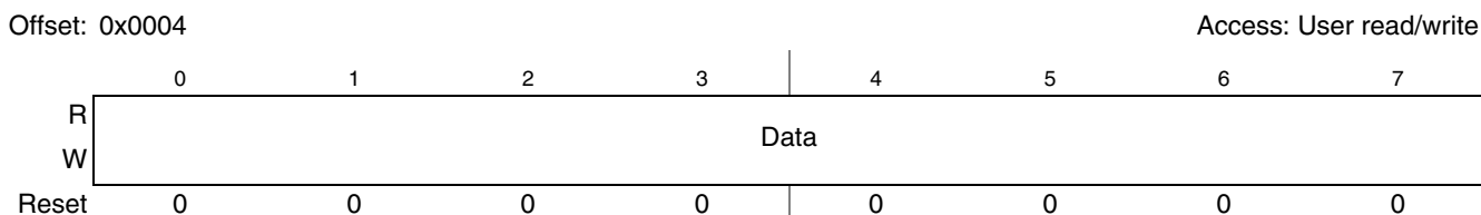
Figure 31-8. I 2 C Bus Data I/O Register (IBDR)
