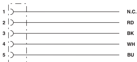
Contact assignment of 7/8" socket
