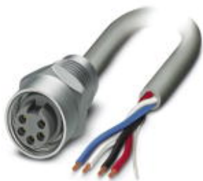
Flush-type connector, 5-position, PVC/PVC, gray, Socket, straight, 7/8"-16UNF, on free cable end, Front mounting, with 1/2 inch-14 NPT mounting thread, Individual wires, cable length: 1 m
