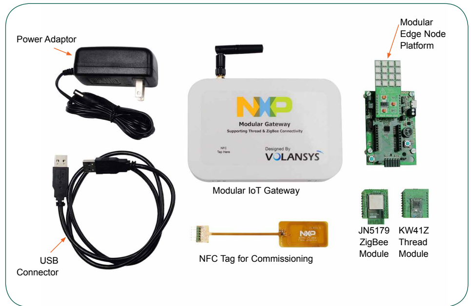
FIGURE 1: SLN-IOT-GPI: IDEx FOR GENERAL PURPOSE IOT SYSTEMS
